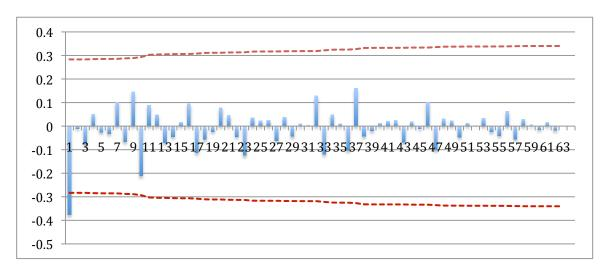
The graph below for the PACF shows critical value lines at plus and minus  $2/\sqrt{n}$ . This seems to indicate pretty clearly that an autoregressive model is appropriate. Given how clearly significant lag one is, a first difference of the data seems unnecessary.
