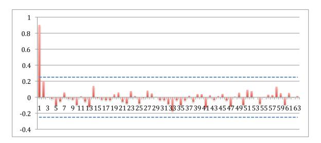
To estimate the model parameters we use the method of moments. Since we have determined that the time series can be modeled with a AR(1), we estimate  $\Phi$  with  $r_1$  which is 0.9018. To estimate the noise variance,  $\sigma_e{}^2$ , we start by estimating the process variance with the sample variance:  $\gamma_0 \approx s^2 = (1/(n-1)) \; \Sigma \; (Y_t - \overline{Y})^2 = 0.7937$ . The noise variance for an AR(1) model is then estimated as  $(1 - r_1{}^2) s^2$  which is 0.1482.
