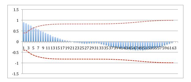
Although the ACF values fall within the error lines by lag 6, they decrease slowly and do not drop to zero. It seems likely that the values could continue sinusoidally for some time. This graph indicates that the series is not based on a moving average formula, or at least not solely on a moving average formula.
